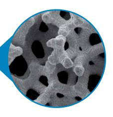
Surgeons provide their patients the closest thing to real bone when using Trabecular Metal Technology. This highly porous biomaterial is designed to replicate the structure, function and physiological properties
